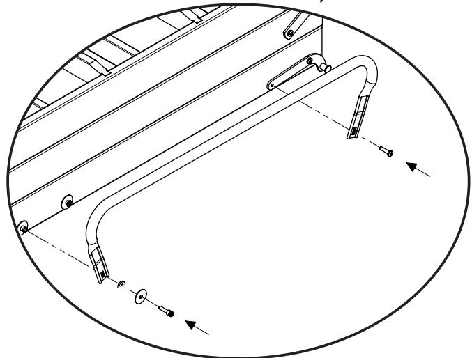
**GB** For ladders where the spring is mounted on to the bracket "a", the spring has to be disengaged before mounting the handrail. Disengaging the spring may only take place when the ladder is in a closed position. Remember to mount the spring again after fitting the handrail.
